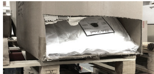
1.1 Creative use of tertiary packaging as storing unit. Part of front has been cut out to ease picking.
